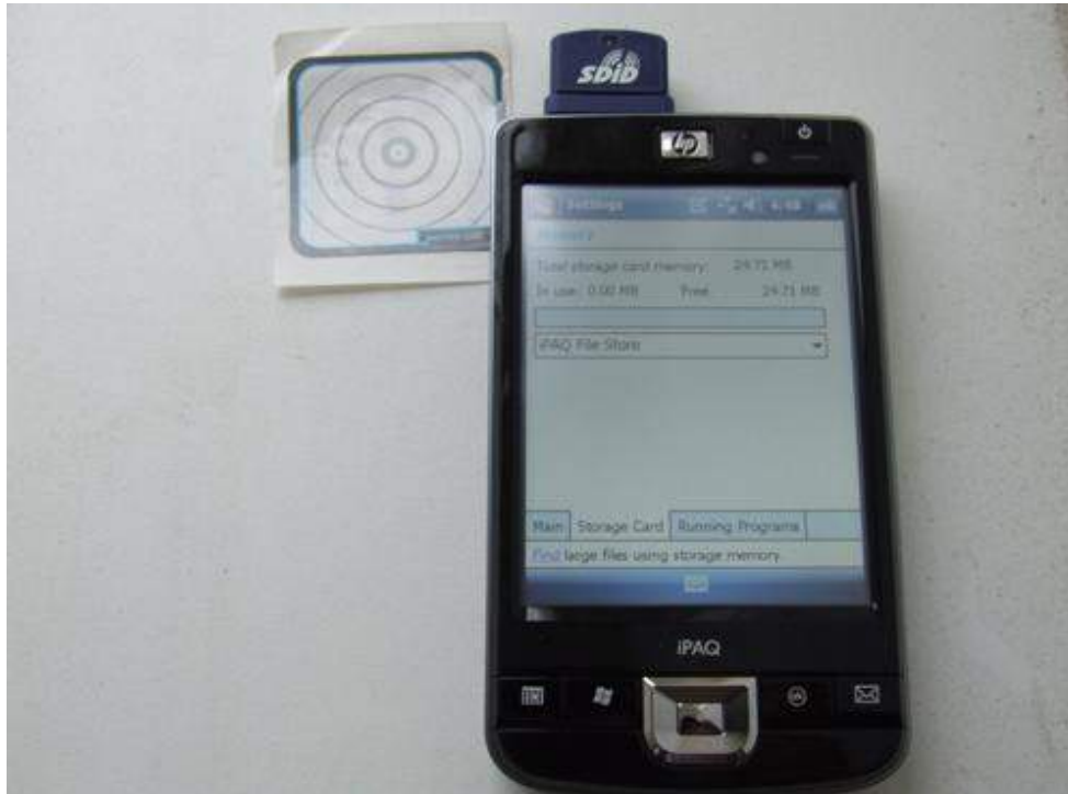
Figure 5 RFID technology test set with HP iPAQ 214 Enterprise Handheld
